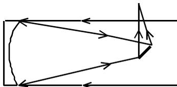
Small reflectors need a *diagonal* mirror to divert light out to the side, so the observer's head won't block incoming light (*Newtonian* design). An eyepiece is used, as with a refractor. A finder scope is needed, preferably a small refractor of straight-through design. A variation on the reflector design is the *Cassegrain*, which has a hole in the objective mirror through which the light is focused.
