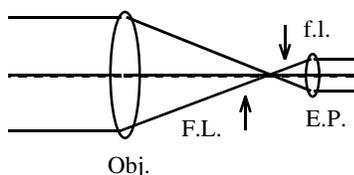
Power is adjusted by changing eyepieces. The shorter the focal length (f.l.) of the eyepiece (E.P.), the higher the power (×).
