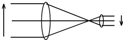
The light rays are made parallel by allowing them to focus and then using a convex lens (in an eyepiece) to straighten them. This gives an *inverted* image, which is usually not a problem.
