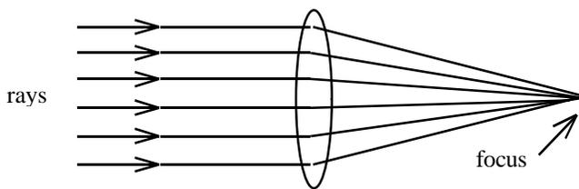
The image may not be viewed directly, since the rays passing through the focal point will diverge; rays must be nearly parallel to be focused by the eye.
